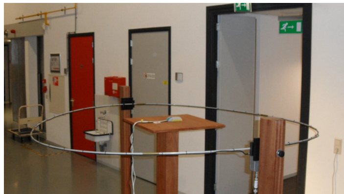
'Radiated emission van Veen loop' test setup (Foto: Dare!!)
