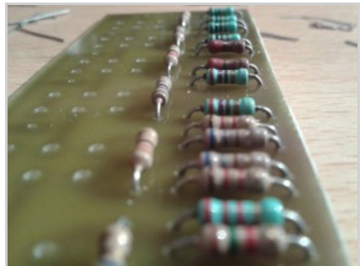
Always start with the resistors.
