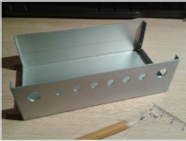
This metal case will hold the circuit (not included in the kit).
